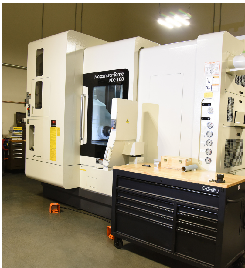
INL recently acquired a 7-axis Nakamura Tome Super MX100 machine. This compact high-precision multitasking machine features a built-in machining and turning center, advanced software, smart features and up to 96 tools.
